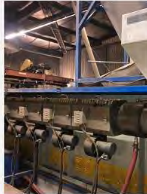
Then melted in an extruder to create plastic pellets...
